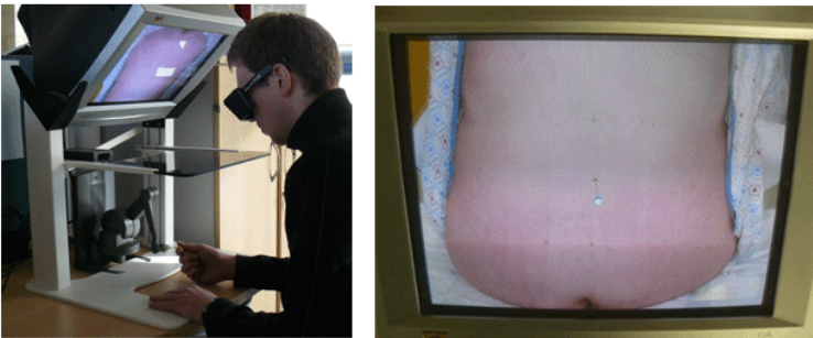
Fig. 3. To the left is a picture of the haptic device in use in the virtual environment and to the right, a screen capture of a patient's back
