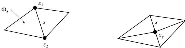
Fig. 12 Patch \omega_s of triangles associated to interior side (left) and its refinement for Dörfler cut-off function (right)
