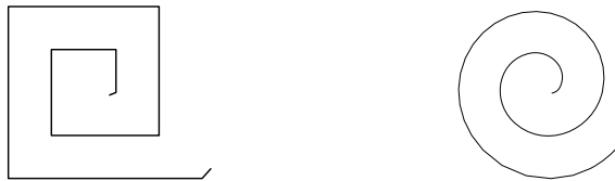
Fig. 7 A control polygon and the limit curve generated by the circle preserving variant of the 4-point scheme
