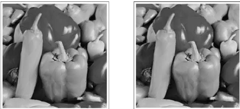
Fig. 9 Approximation by 2000 anisotropic triangles obtained by the greedy (left) and modified (right) algorithm
