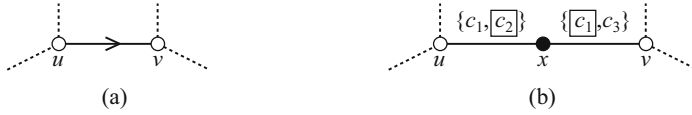
Fig. 3. (a) an NCL edge uv and (b) its corresponding edges ux and xv of a graph with lists L(ux) = \{c_1, c_2\} and L(xv) = \{c_1, c_3\}
