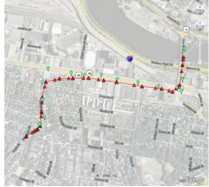
(b) Estimating a trajectory using the map. Each prediction is indicated by a triangle, while each measurement is drawn as a balloon. The predicted trajectory is shown in solid lines.
