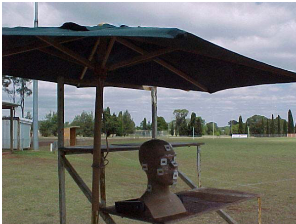
Figure 7.1 A human form manikin with dosimeters placed at various anatomical sites measuring the UV protection provided by a shade umbrella
