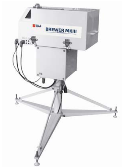
Figure 6.2 Photograph of the Mark III version of the Brewer Spectrophotometer (Courtesy of Kipp and Zonen)
