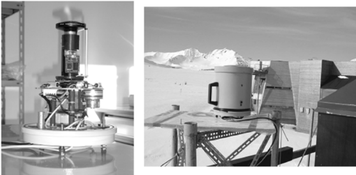
Figure 4.11 Total Sky Camera (TSC); inside view and outdoor location
