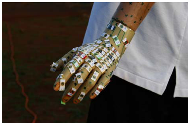
Figure 7.2 UV exposure measured by application of miniaturized polysulphone dosimeters placed on the hand of a life-sized manikin
