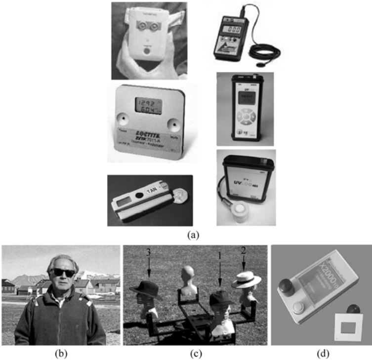
Figure 4.18 (a) Commercial electronic dosimeters; Examples of personal dosimeters; (b) Rafanelli et al. 2002; (c) Kimlin and Parisi, 1999; (d) Electronic dosimeter and dosimeter badge by polysulphone film
