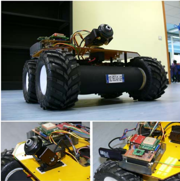
Fig. 7. A wheeled robot, with an integration of our generic vision system. The webcam moves with two motors, managed by the control module shown on the last photo.
