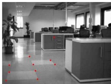
Fig. 9. Some Augmented Reality content inserted on what the teleoperators can see: here, the ground analyze and a target to reach (red points)
