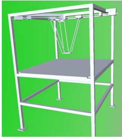
Fig. 5. TRIGLIDE Virtual Reality model made in Matlab/Simulink
