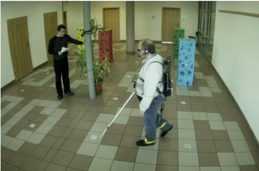
Fig. 3. Navigational trials were automatically recorded. Markings on the participants' pant legs and on the floor allowed precise path reconstruction.
