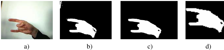
Fig. 1. (a) – input picture, (b) – picture after binarization based on skin colour, (c) – image after applying morphological operations and the choice of the largest object, (d) – hand image after centering and scaling into 64x64 pixels
