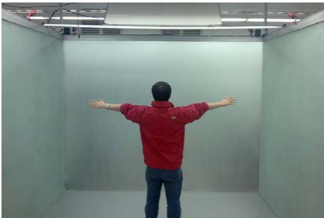
Fig. 14. The actual setting of the imseCAVE. Infra red cameras are attached at the top of the imseCAVE
