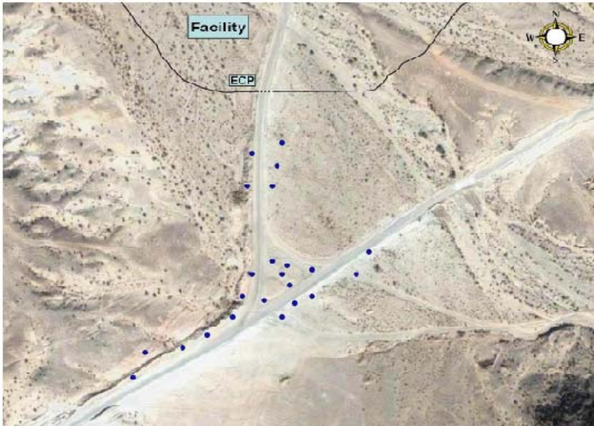
Fig. 3.2 Vehicle Tracking Scenario Map. Blue dots are seismic/acoustic sensor nodes. The speed, heading, location, and vehicle type are estimated by independent CARTMAP networks using binary data from all sensor nodes as input
