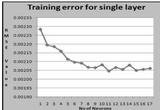
Fig. 3. The training error of the single layer ANN plotted against the number of neurons used in the hidden layer
