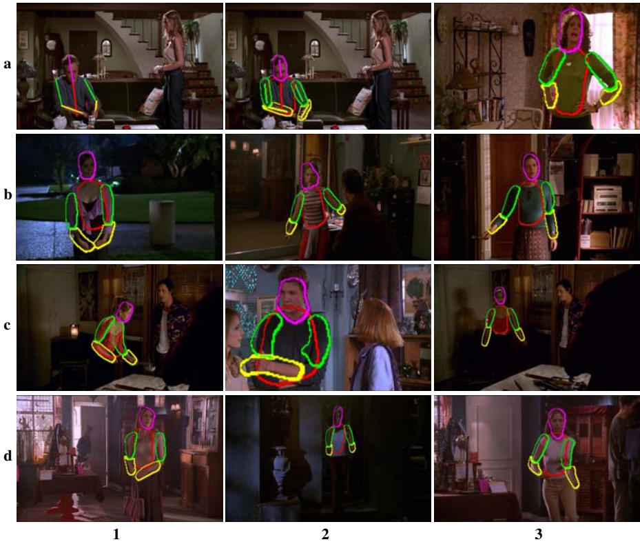
Fig. 10. Pose estimation results I. (a1) example ground-truth ‘stickman’ annotation. All other subfigures are the output of the proposed method, with body part segmentations overlaid. For illustration, in (a2) we also overlay the stickman derived by our method. The color coding is as follows: head = purple, torso = red, upper arms = green, lower arms = yellow. In (c2) a pose with crossed arms is correctly estimated: the repulsive model does not prevent our system from dealing with these cases.
