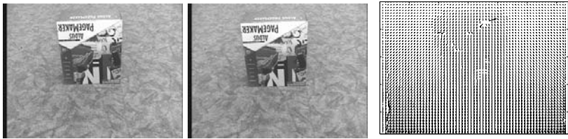
Fig. 12. Same as Fig. 11 but for the image sequence with obstacles. The images I(t) and I(t + 1) and the optical flow field \mathbf{u} are used for the detection of the ground plane.
