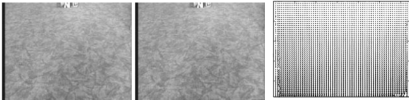
Fig. 11. Model Image Generation Left and Middle: image sequence without obstacles. The pair of images is successive image I_m(t) and I_m(t + 1) for the computation of the optical-flow model. Right: optical-flow model \mathbf{u}_m .
