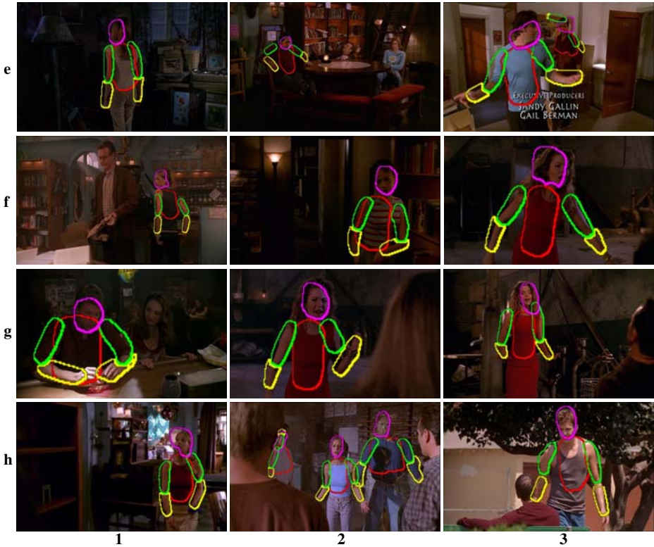
Fig. 11. Pose estimation results II. More example pose estimations. A fair sample of failures are also included, e.g. (f1) is missed as a detection, and the wrong pose is obtained in (e3) (rear person). Notice how the leftmost person in (h2) is largely occluded.
