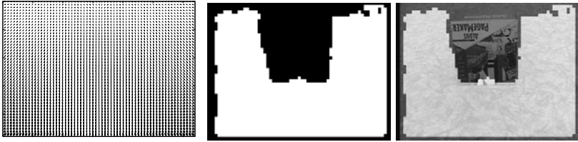
Fig. 14. Dominant plane detection by temporal model-based method Left: planar flow. Middle and Right: dominant plane. The dominant plane is detected by the temporal-model-based method. The white and black regions represent the ground plane without obstacles and that with obstacles, respectively.
