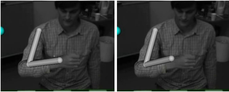
Fig. 13. Noise of the 3D Body Tracker. The two consecutive frames show the estimated arm by a 3D body tracker [3]. The estimation is in this specific experiment not very accurate (noisy).
