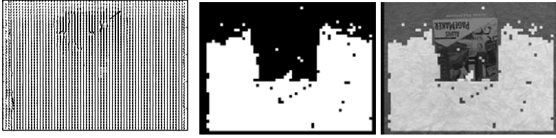
Fig. 13. Dominant plane detected by model-based method. Left: observed optical flow. Middle and Right. dominant plane The white and black regions represent the ground plane without obstacles and that with obstacles, respectively.
