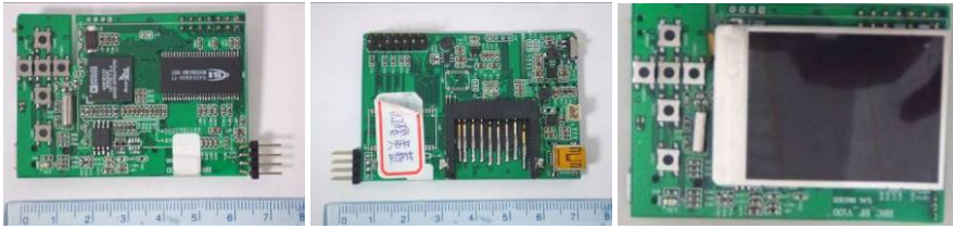
Fig. 4. The Picture of DSP Platform (Dimension: 64 x 45 mm 2 )
