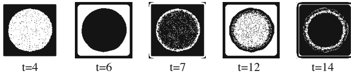
Fig. 4. Simulation results of the segmentation by a conventional method using PCNN. The input image is gray-scaled image (only intensity of the image is considered) which is shown in fig 3(a). No characters or significant segments are shown in any time step.
