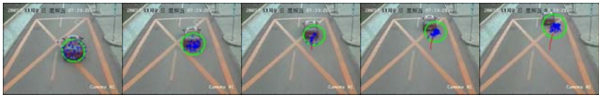
Fig. 5. Traditional particle filtering tracking (Frames 10, 24, 39, 56, and 60 are displayed)
