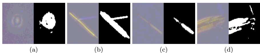
Fig. 11. Example of false positive. (a) an air bubble (b) an overlap of particles (c) a decoupling by the out of focus (d) a fiber with broken pieces
