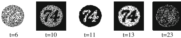
Fig. 6. Simulation results of the segmentation by our proposed IC-PCNN. The input image is full color image. The target character "74" is segmented as shown in several time steps.
