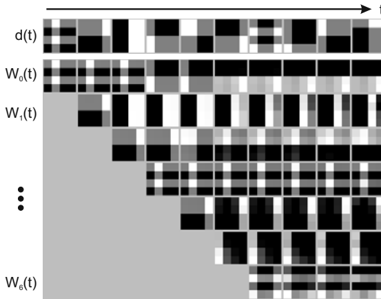
Fig. 5. While provided with the first ten images (top), the iNMF algorithm generates seven base vectors (bottom). The first seven input images are simply stored one-to-one in the base vectors. After this phase, the base vectors are adapted and become less complex and sparser.
