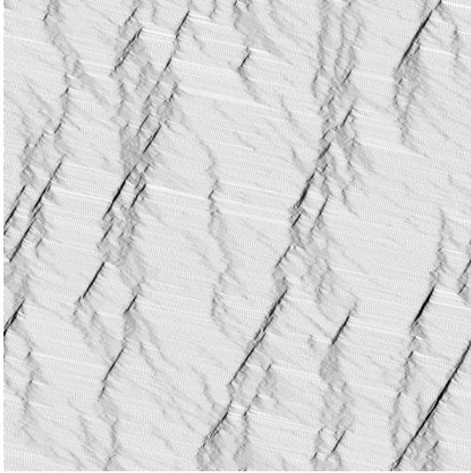
Fig. 3. A 'zoomed-out' view of a larger simulation of our 'slow-to-stop' model. Black dots refer to cars, while white space is empty road. The simulation parameters used to produce this output are the same as those used for Figure 2. Cars drive from left to right, and time 0 is at the top.
