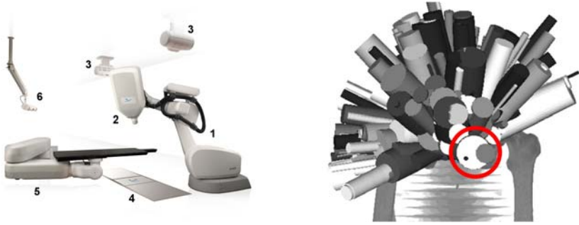
Fig. 1. The robotic CyberKnife system by Accuray Inc. The system consists of a robotic arm (1), linear accelerator (2), X-ray sources (3) and orientation, diameter, and weight of the beams cameras (4), a robotized patient couch (5), and an optical tracking system. (Image courtesy of Accuray Inc.)
