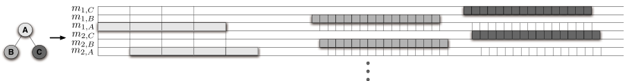
Fig. 3. An example of the reduction with r = 2, d = 2, I_1 = \{A\} and I_2 = \{B, C\} . Only the two first out of r^{2d} = 16 groups of machines are depicted with the jobs corresponding to A, B , and C to the left, center, and right respectively.
