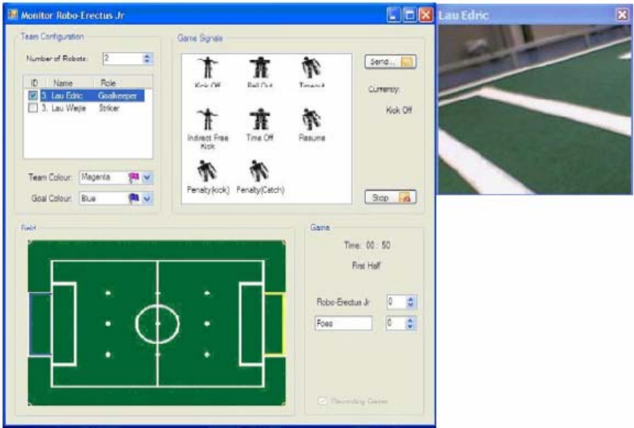
Fig. 3. Human Robot Interaction System of Robo-Erectus Junior Humanoid Robot
