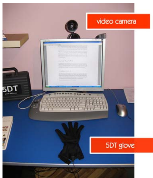
Fig. 7 Gesture acquisition scenario: video camera points down toward the desk tracking the user’s hand; a 5DT sensor glove detects finger flexion
