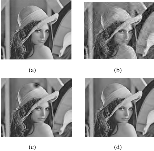
Fig. 11 Subjective quality of decoded ‘Lena’ image at 0.1 bpp and CNR=20 dB (a) original image (b) with QAM (c) with H-QAM for \alpha=1.5 and (d) with H-QAM for \alpha=1.8
