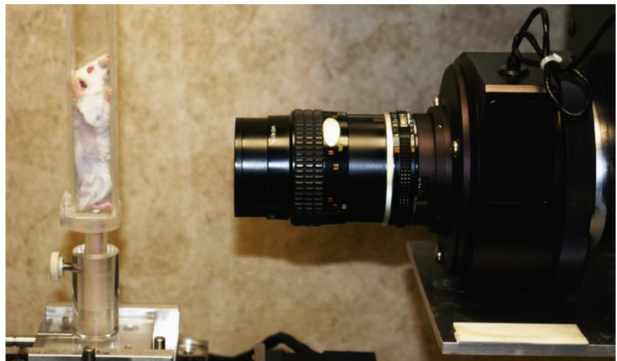
Fig. 9.2 Basic bioluminescence imaging (BLI) system used in the first BLT system with a cooled charge-coupled device (CCD) camera, a Nikon 55 mm lens, and a rotation mouse stage
