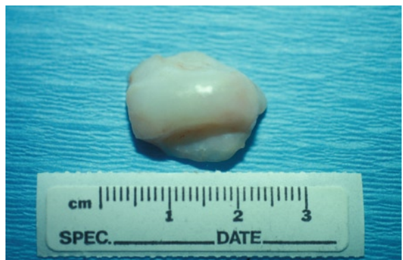
Fig. 26.16 Temporomandibular joint disc replacement created by tissue engineered growth of chondrocytes in an animal model
