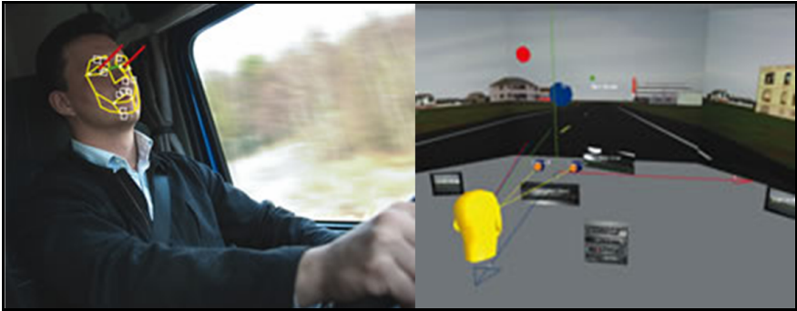
Fig. 1. Tracking of a subject's gaze with free head movement in a 3D environment
