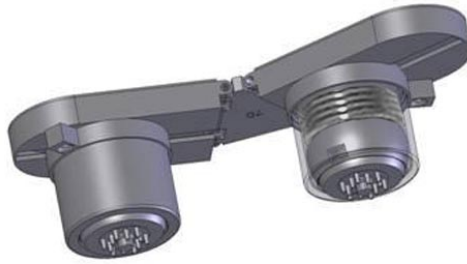
Fig. 2. Illustration with an internal view of the sensor enclosure design that fits within a Navy flight helmet above the ear cup with spring-mounted optics that allow for self-rotation of the optical components
