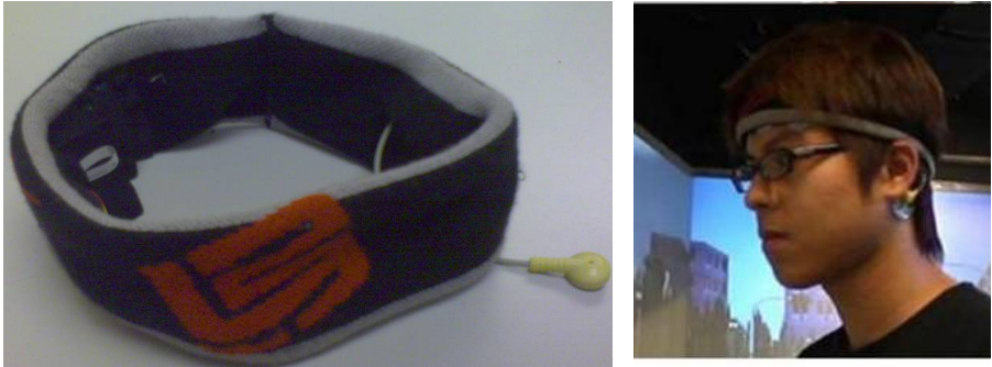
Fig. 3. A picture of the wearable & wireless EEG system, NCTU BCI-headband. It comprises 4- or 8-channel snap-on electrode holders (plus a reference and a ground channels), miniature bio-amplifier, a bandpass filter, an ADC and a Bluetooth module. All channels were referred to the left mastoid.
