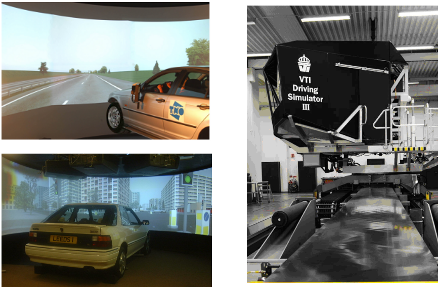
Fig. 1. The driving simulators used in the experiments. Top left, the TNO simulator; bottom left, the (old) ITS Leeds simulator; right the moving base driving simulator at VTI.
