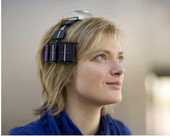
Fig. 3. Autonomous wireless EEG system powered by body heat and ambient light
