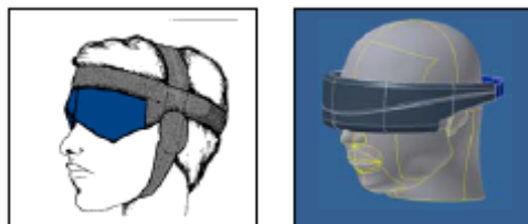
Fig. 6. Two potential form factors: a soft ski-mask design (left) and a more rigid visor design (right). In both cases the electronics and batteries will be housed in the appropriately designed eye cover.
