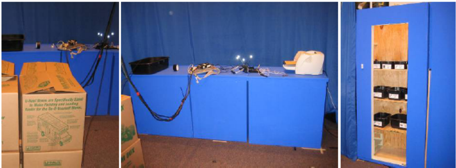
Fig. 1. In the physical environment, we have a combination of chroma-key blue material objects and visible objects. The chroma-key allows overriding the appearance of real objects, enabling the patient to believably touch virtual surfaces.
