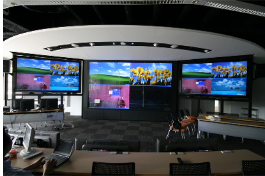
Fig. 2. CDF (Concurrent Design Facility) system. This system consists of 4K stereo projector and two LCD monitors.
