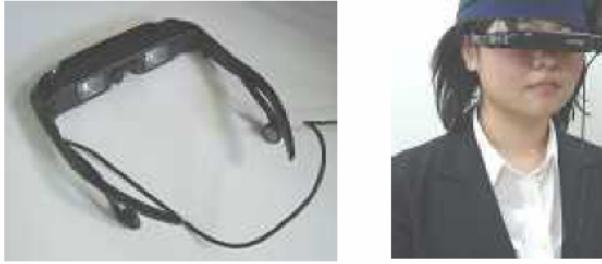
Fig. 1. An HMD (iWear AV920, Vuzix Corporation; 640x480dot) used in the present experiment
