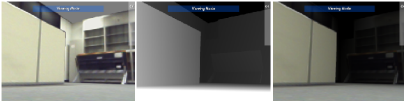
Fig. 4. Examples of PTM (left), depth mapping (center), and mixed mapping (right)
