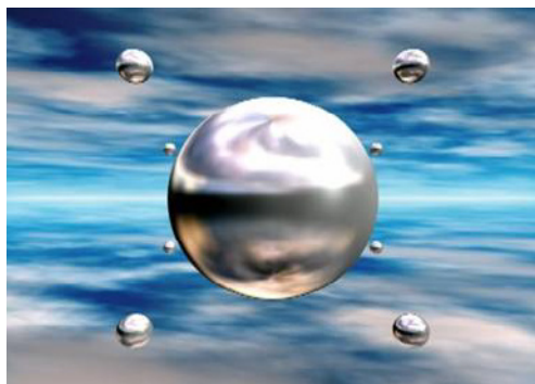
Fig. 1. An image produced using the POWER-3D method. The next image for the other eye is laterally shifted by a few centimeters due to the angle of convergence. An observer using glasses with liquid crystal shutters perceives the images in three dimensions.
