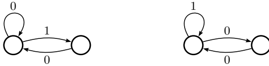
Fig. 2. Finite automata for the G -shift (left) and for the (-G) -shift (right)
