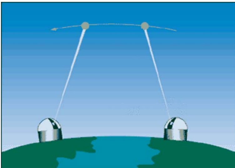
Fig. 2.7. Principle of satellite laser ranging.
