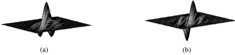
Fig. 1. (a) The real part and (b) the imaginary part of a Gabor filter
