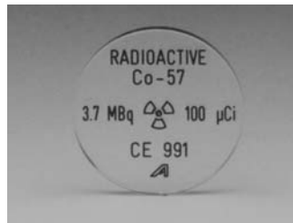
Figure 7.2 Pointlike emitter, in this case 3.7\text{ MBq }^{57}\text{Co} , for use in the field of radiography (type 25/3, AEA Technology QSA GmbH)
