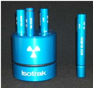
Figure 7.1 Design-approved radioactive sources for demonstration experiments (QSA Global GmbH)
