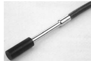
Figure 10.8 Diamond detector as solid-state ionization chamber for the relative dosimetry of X rays and beta rays; measurement range 80 keV–20 MeV for photons, 4–20 MeV for electrons (PTW–Freiburg, Germany)
