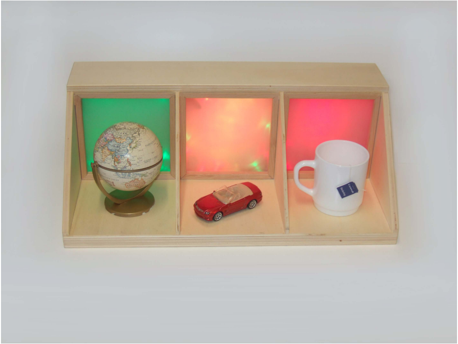
Fig. 1. The ambient display subsystem of the Tangible Reminder, with an object in each tray, showing the different colors for different states
