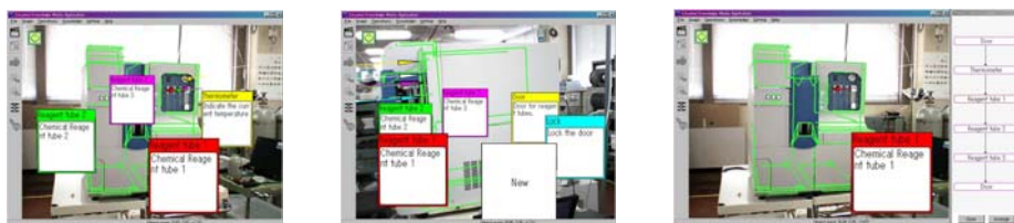
Fig. 4. Example of the current AR interface. The EMGA unit is augmented with SKQs. The green model superimposed on the image is useful for the user to determine if the object recognition result is correct. Each SKQ (colored box) is only partially shown, it has to be selected so as to be fully displayed. The right image shows a procedure in which each step represents a particular SKQ.
