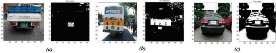
Fig. 3. Vehicle image LP and its color segmentation results using HSI color model
