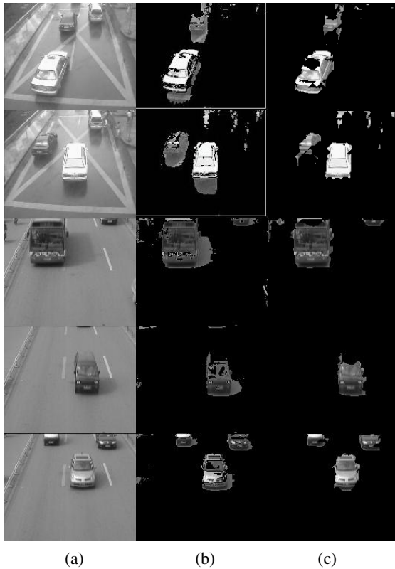
Fig. 9. Shadow elimination (a) original frames; (b) extracted foregrounds; (c) foregrounds after shadow elimination
