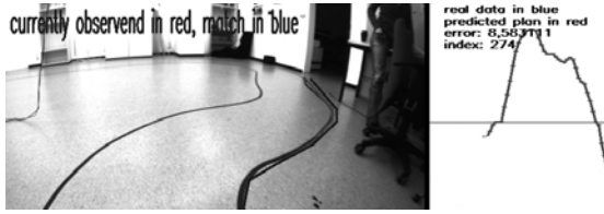
Fig. 4. Screenshot example of the planner operating mode. Left: The observed street (gray, originally red) is compared to the database entries and the best match is returned (black, originally blue). Right: The assigned steering sequence of the best match.
