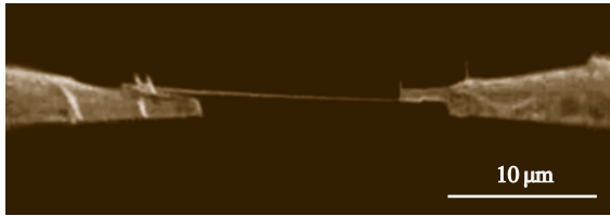
Fig. 7.16 Electron biprism fabricated by FIB-CVD
