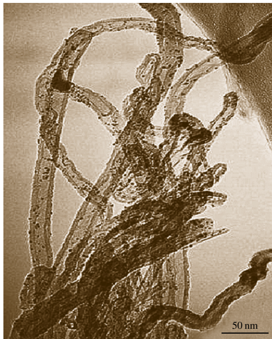
Fig. 3.31 Transmission electron microscopy image showing rhodium nanoparticles supported on the surface of an MWNT (from [3.329]) ▶
