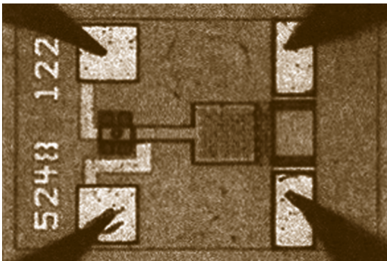
Fig. 12.47 Top view photo of a fabricated metal-to-metal contact switch (after [12.49])
