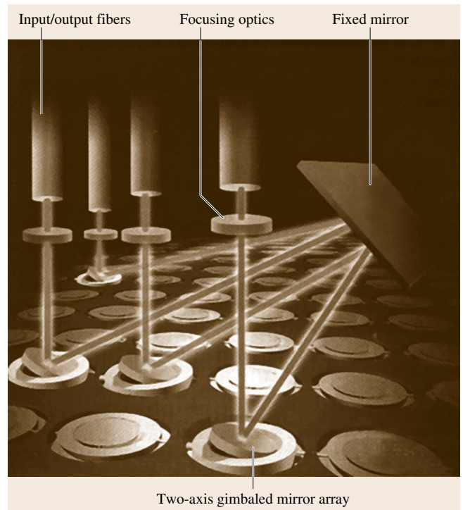
Fig. 12.31 Schematic of a three-dimensional micromirror-based fiber optic switching matrix
