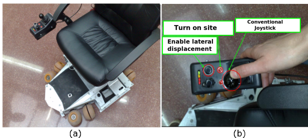
Fig. 1. (a) Holonomic wheelchair Spherik, by ESCLATEC. (b) Spherik joystick and controls to turn.
