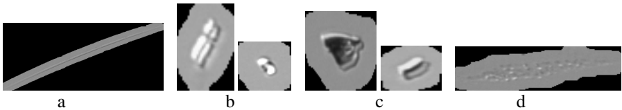
Fig. 3. Images of characteristic items: a) scratch; b) dig; c) dust; d) cleaning marks
