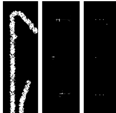
Fig. 4. Centre from events algorithm applied to a path
