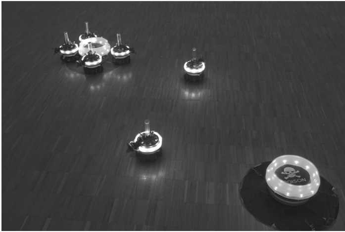
Fig. 2. Robots are positioned in an arena with a food object and a poison object that look the same at distance. Robots can communicate by changing color and by observing the color of the surrounding robots. The picture shows an evolved group of four robots feeding on the food object positioned in the top left corner while they are lighted up in blue color. Two robots in white color are attracted by the blue signal and move away from the poison object positioned in the bottom right corner.
