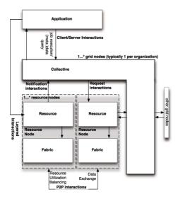
Fig. 1. Structural View of the Grid Reference Architecture
