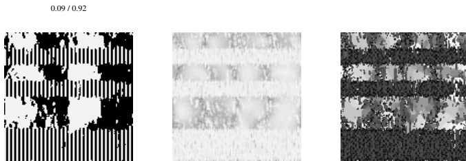
Fig. 3. Segmentation result of the maximum membership rule is on the left, in the middle is an image of the confidences at each location, and the right image gives the local scales (white equals 24, black \frac{1}{2} ). The numbers in the title of the left image gives the error and the average confidence, respectively.
