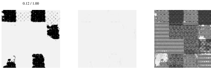
Fig. 6. Segmentation result of the maximum membership rule is on the left, in the middle is an image of the confidences at each location, and the right image gives the local scales (white equals 24, black \frac{1}{2} ). The numbers in the title of the left image gives the error and the average confidence, respectively.
