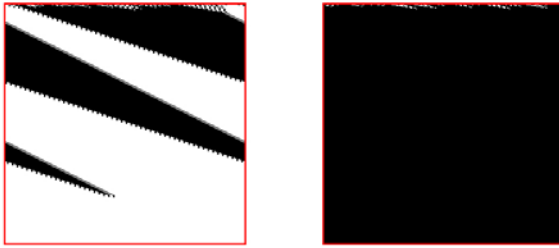
Fig. 1. The evolution of a CA for a 0s block-expanding rule (011200000000A57F7FFFFDF777FFFF) with a performance of 0.6485 and a fitness of 0.98. On the left, the density of 1s is less than 1/2 while, on the right, the density of 1s is higher than 1/2 .
