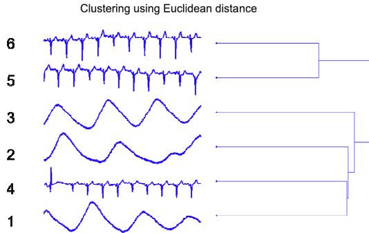
Fig. 2. Result of hierarchical clustering using Euclidean distance on raw data. In fact, using DTW produces the same result.
