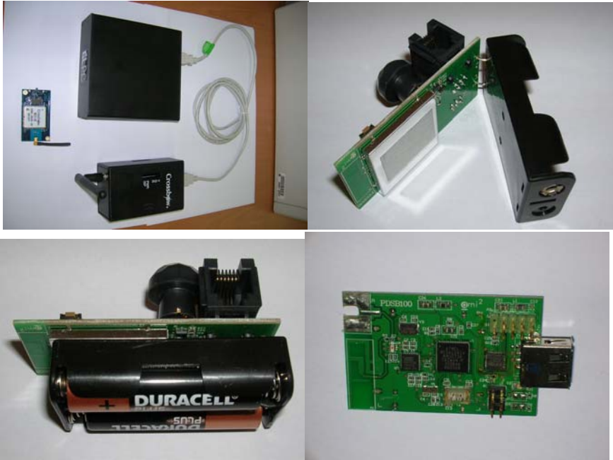
Fig. 4. Gateway based on miniPC, Mote board and base station
