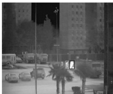
Fig. 4. Selected image with two objects of interest: a person is bounded by a white box and a fire is bounded by a black box
