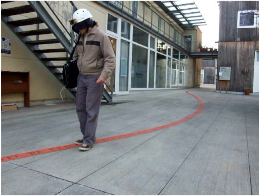
Fig. 2. A blindfolded individual following a coloured sinuous path with a head mounted webcam and a notebook carried in a shoulder pack
