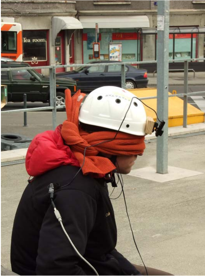
Fig. 1. A webcam prototype worn by a blindfolded participant (headphones are not visible)
