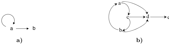
Fig. 1. In a) , it is presented the graph representation of the argumentation framework: \langle\{a, b\}, \{(a, a), (a, b)\}\rangle . In b) , it is presented the graph representation of the argumentation framework: \langle\{a, b, c, d, e\}, \{(a, c), (c, b), (b, a), (a, d), (c, d), (b, d), (d, e)\}\rangle .
