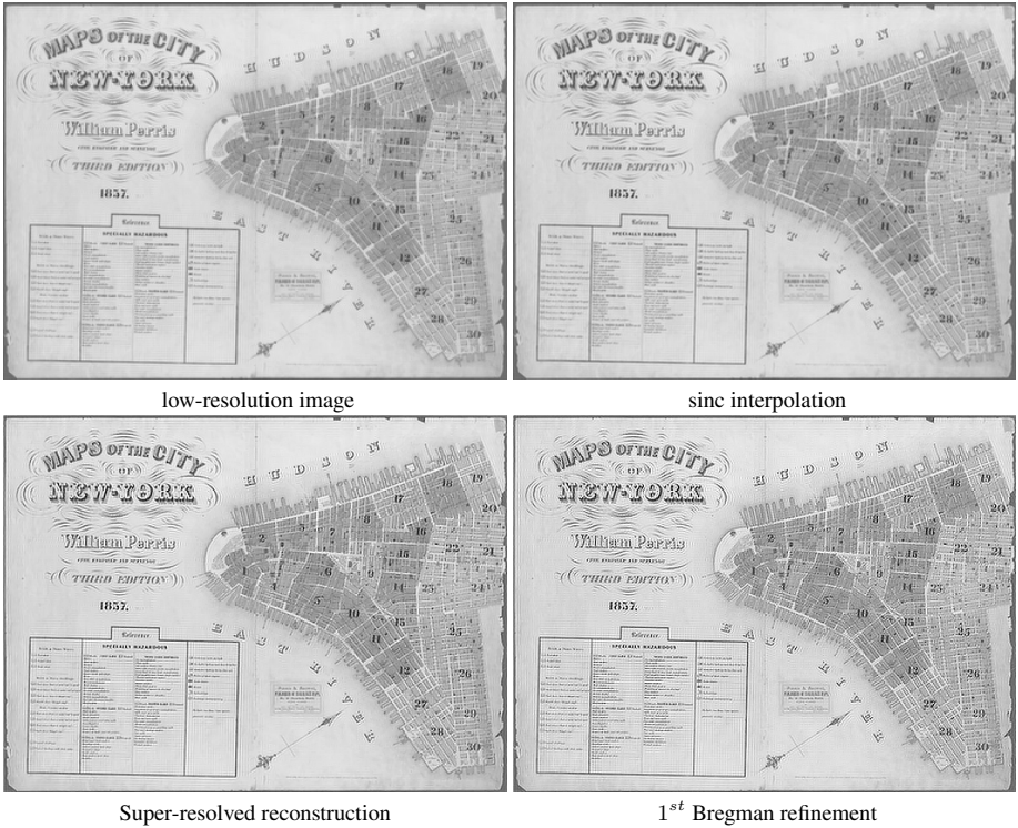
Fig. 2. Clockwise from top, a 380 \times 285 low-resolution image, upsampled to twice the size by sinc interpolation, and super-resolved reconstruction, and the first Bregman iterated image
