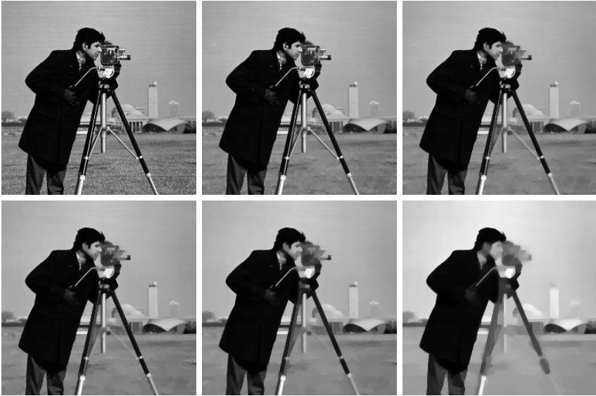
Fig. 4. Influence of the smoothness parameter \theta . First row: original image and smoothed images with \theta = 0.55 and \theta = 0.60 . Second row: smoothed images with \theta = 0.65 , \theta = 0.70 , and \theta = 0.80 .
