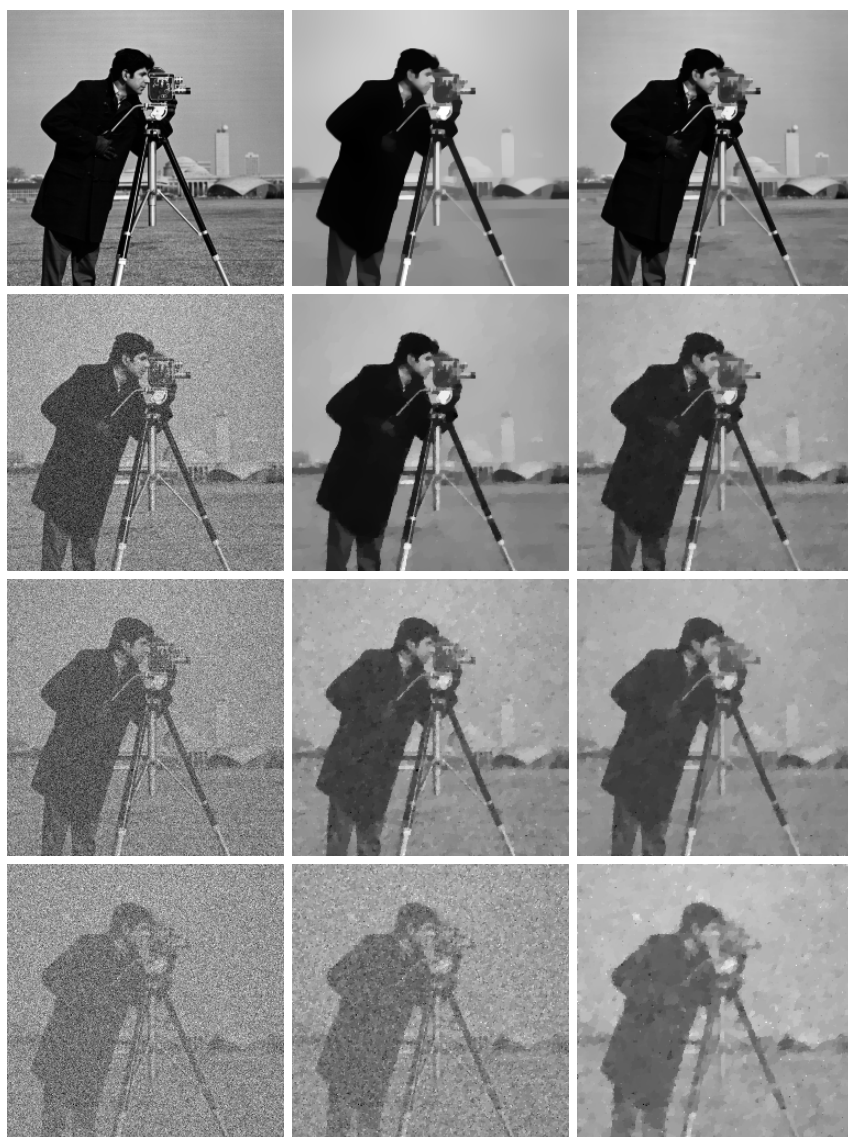
Fig. 3. Left column: image with Gaussian noise; the noise level increases with each row ( \sigma = 0, 30, 50, 100 ). Middle column: total variation denoised image with constant parameter choice. The regularization parameter is kept the same for all images. Right column: denoised images with adaptive parameter choice for a smoothness parameter \theta = 0.60 .
