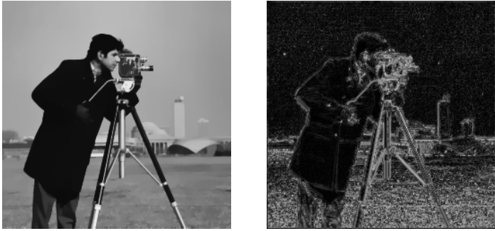
Fig. 1. Smoothed image (left) and corresponding function \Sigma_r (right). Bright pixel values indicate a higher value of \Sigma_r .
