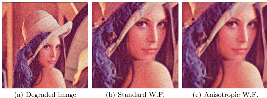
Fig. 4. Color image degraded by a gaussian kernel and uncorrelated Gaussian noise (4(a)) with standard deviation of 10%. Figures 4(b) and 4(c) show the results for the standard and the anisotropic reconstruction.
