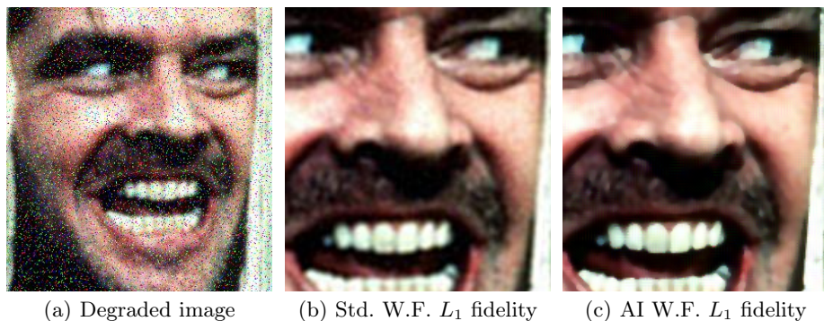
Fig. 5. Color image degraded by a gaussian kernel and uncorrelated impulse noise (5(a)) with density 0.11. Figures 5(b) and 5(c) show the results for the standard and anisotropic restoration based on the L_1 fidelity term.
