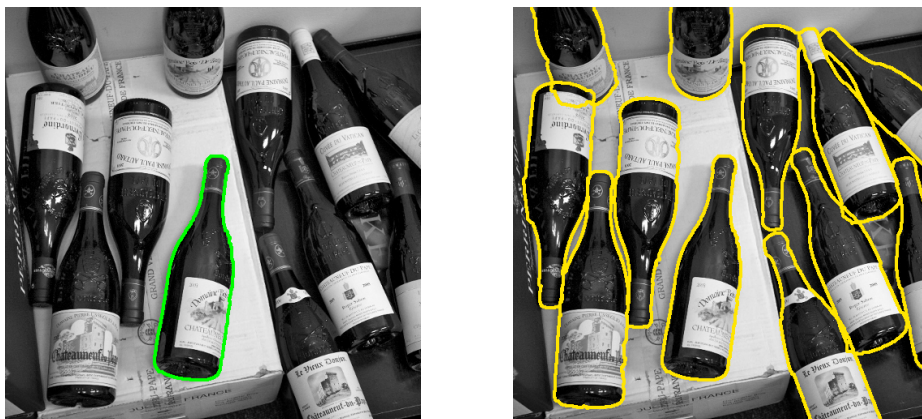
Fig. 9. Segmentation of bottles with a single shape prior
