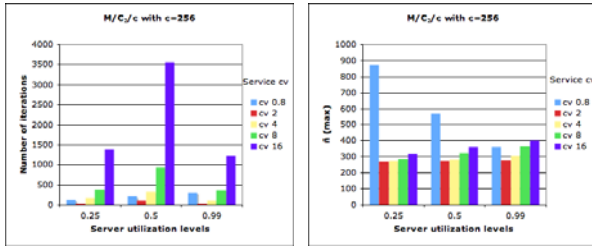
(g) Number of iterations with 256 servers. (h) Maximum value of \tilde{n}^i with 256 servers.
