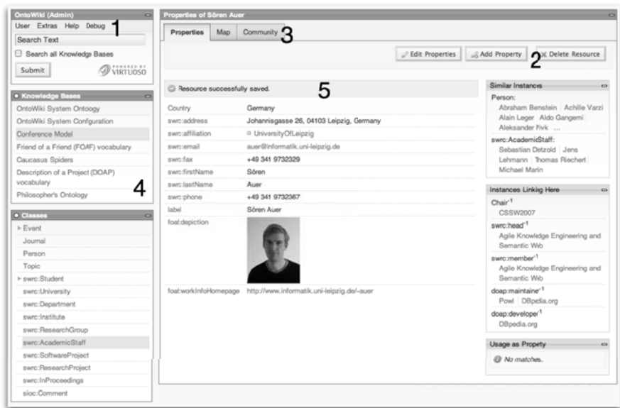
Fig. 3 Screenshot of OntoWiki with OntoWiki Application Framework components: 1) menu, 2) toolbar, 3) navigation, 4) module window and 5) message
