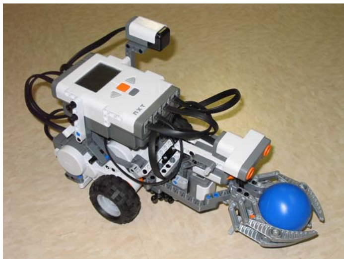
Fig. 5. A picture of the ARCHIE MINDSTORMS robot: a three-wheeled design with a grasping arm and a number of mounted sensors along with the NXT processor brick
