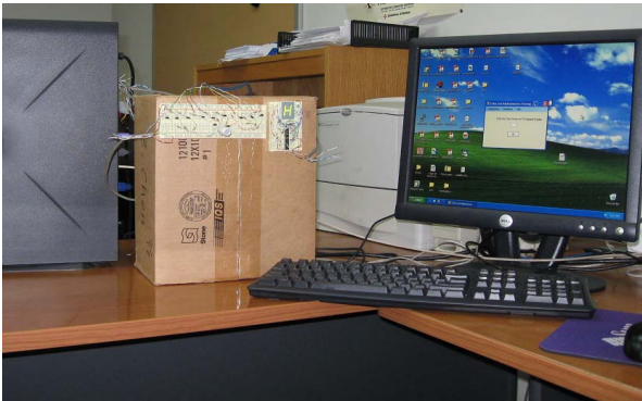
Fig. 2. Overall Experimental Setup of the Color and Alphanumeric Pairing (the cardboard box with the multi-color LED and the SSD, simulates, e.g., an access point in a cyber-cafe; the desktop simulates the laptop.)
