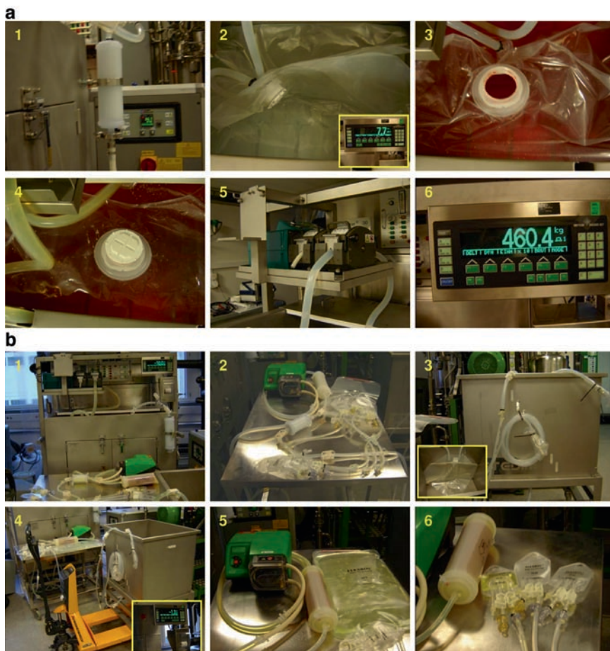
Fig. 6.a Preparation of 500-L media. Mixing station (1) and the 0.1-mm filter for bioburden control of the added WFI water used for media preparation. In the back is the mobile temperature control unit of the mixing station. Media preparation manifold (2) placed inside the mixing station. The water volume added is controlled by weight. Spout (3,4) used for the addition of the media components. This spout is closed during mixing through recirculation using peristaltic pumps (5). The volume is controlled through weight during media preparation. b Various steps for media dispensing after preparation. The 500-L mixing station (1) with the prepared media. The peristaltic pump (2) used to dispense the media from the preparation bag to the storage bag, the 0.2- and 0.1-mm filters, the flush bag for the filters and the quality control (QC) sampling bags, respectively. Empty storage bag (3,4) placed in a steel vessel that is itself located on a jack lift with an integrated scale for weight control. Flush bag (5,6) for the filters and the QC sampling bags, respectively
