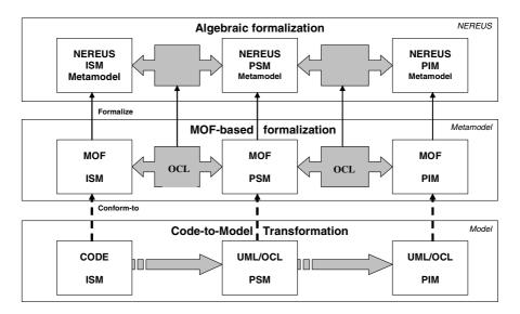
Fig. 1. A framework for MDA-based reverse engineering
