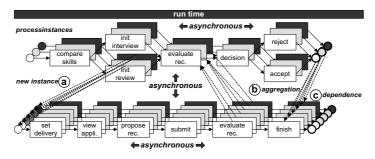
Fig. 5. Synchronizing process instances
