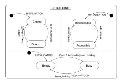
Fig. 10. Concurrent state/transition diagram of class BUILDING
