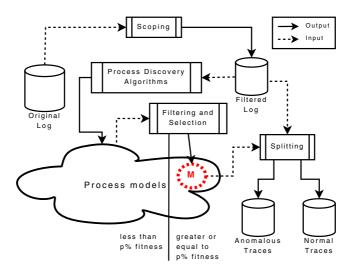
Fig. 1. Overview of our anomaly detection approach
